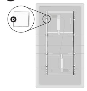
**NOTE:** If placing base on top of a bed with slats, ensure non-skid pads are spaced according to slat location.
