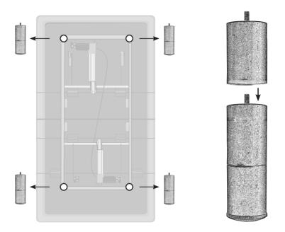
Position bars A along either side of the base so that the correct holes are aligned with the existing legs. Secure bars A to base using screws allen wrench C.
